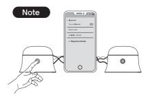
While the speakers are in TWS pairing mode, you can press and hold the button on either one to shut both of them off.
