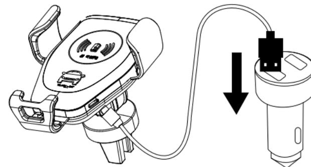
1. Connect Micro-USB charging cable to wireless charger.
